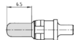
Premating plug contact
