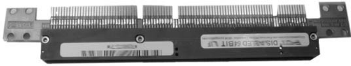
↑ 64 Bit 5V PCI Connector mounted to PCI Bus Extender Card.
