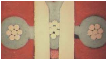
Cross section ribbon cable AWG-26 stranded wire 180° cable outlet
